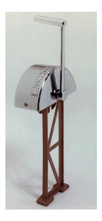
Model 2093 remote control for model 2091 is of the same rugged design. Entirely made up of die cast silicon bronze and stainless steel hardware and is backed with our usual warranty. This head comes with all the hardware to mount the interconnecting cables. These must be 47 series pull/pull cables.
