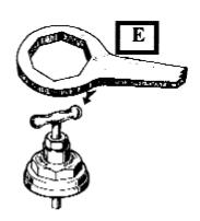
Withdraw the pump assembly.
