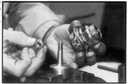
ASSEMBLE IN REVERSE ORDER. NOTE: APPLY SEMI-HARDENING JOINTING COMPOUND TO THE THREADS ON THE LOWER VALVE HOUSING.
