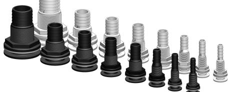
The Skin Fitting with Tail body and nut are moulded from glass fibre reinforced nylon composite. High strength, high-modulus glass fibres impregnated into the nylon provide dramatic strength, stiffness, toughness and dimensional stability. These properties allow a significant weight reduction over metallic fittings.
