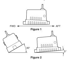
It is important that the switch is mounted 1/4" (6mm) above the bottom of the pump strainer. This will assure a positive shut off of the pump.
