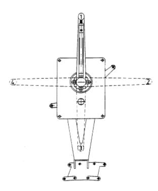
This control can be **ordered** (can not be changed in the field) with the neutral position of the handle in any one of the four positions indicated. Position "1" is standard. Please add appropriate number.
