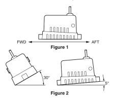
It is important that the switch is mounted 1/4" (6mm) above the bottom of the pump strainer. This will assure a positive shut off of the pump.
