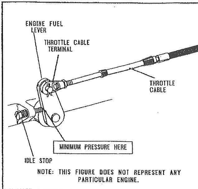
FIGURE 6 THROTTLE CONNECTION
