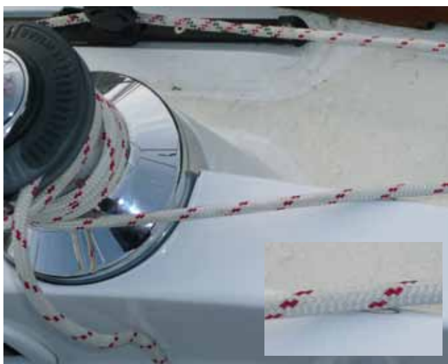
Before: The rope burns through the coaming
