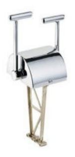
This control is available with three different handles; standard, handles with plastic grips or curved handles with knobs. An optional clutch and throttle interlock can be ordered with this unit. The purpose of this interlock is to prevent shifting, above engine idle. It is only available for systems having clutch and throttle on the same control. In two station applications only one interlock is required. For gears with an electric clutch, an adapter with two microswitches can be ordered.
